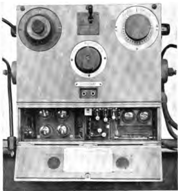
FIG. 201 a.—Telefunken 10 watt C.W. aeroplane or ship set. [To face p. 404.]
